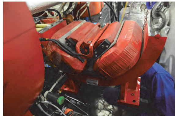
Fig. 2. The sextupole main coil wound on the pole face of a quadrupole magnet.
